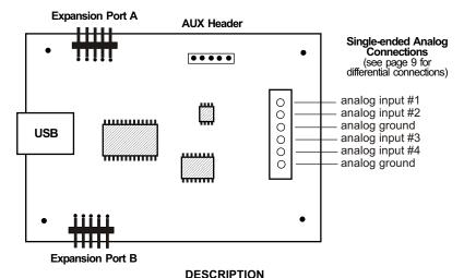
The ADC-4U series Analog to Digital converters connect to any available USB port on your desktop or laptop PC (including some tablets and phones). Four analog inputs channels are provided for conversion to 8, 10 or 12 bit digital format. The converters may be set to two channel fully differential mode if required. Three optional expansion ports are available for connection of up to 144 relays, 144 status inputs or combinations of relays and inputs.
